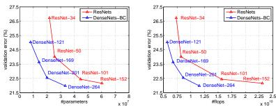
**Figure 3:** Comparison of the DenseNets and ResNets top-1 error rates (single-crop testing) on the ImageNet validation dataset as a function of learned parameters (*left*) and FLOPs during test-time (*right*).
