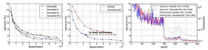
**Figure 4:** *Left:* Comparison of the parameter efficiency on C10+ between DenseNet variations. *Middle:* Comparison of the parameter efficiency between DenseNet-BC and (pre-activation) ResNets. DenseNet-BC requires about 1/3 of the parameters as ResNet to achieve comparable accuracy. *Right:* Training and testing curves of the 1001-layer pre-activation ResNet [12] with more than 10M parameters and a 100-layer DenseNet with only 0.8M parameters.
