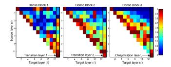
**Figure 5:** The average absolute filter weights of convolutional layers in a trained DenseNet. The color of pixel  $(s,\ell)$  encodes the average L1 norm (normalized by number of input feature-maps) of the weights connecting convolutional layer s to  $\ell$  within a dense block. Three columns highlighted by black rectangles correspond to two transition layers and the classification layer. The first row encodes weights connected to the input layer of the dense block.
